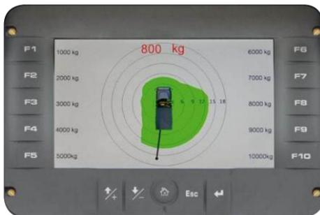
**Crane lifting capacity always under control in all stabilizer positions.**
