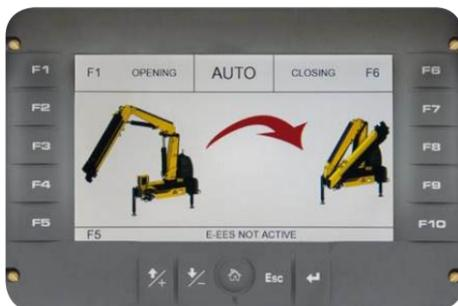
**Crane Automatic folding/unfolding.**
